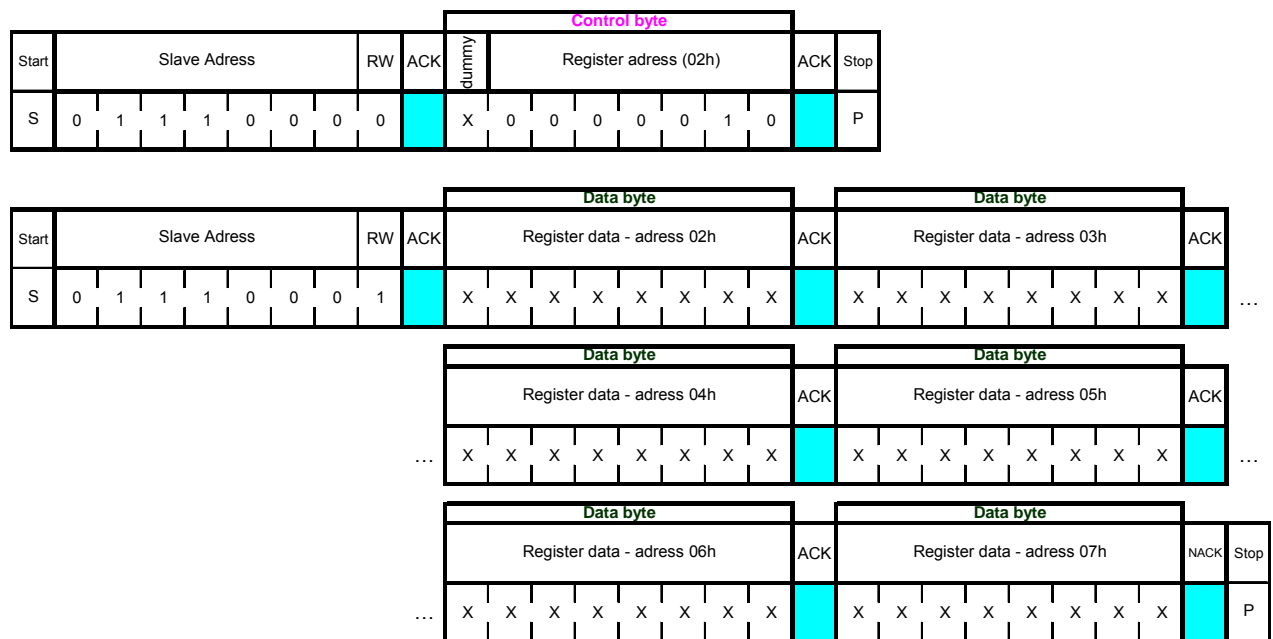
Figure 16: I 2 C multiple read protocol. Address register is first written to BMA020, the RW=0 (lowest acceleration data located at address 02h). I 2 C transfer is stopped and restarted with RW=1, address is automatically incremented and the 6 bytes can be sequentially read out.
