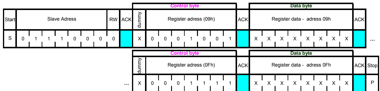
Figure 15: I 2 C multiple write protocol
